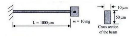
Figure 1.(A beam spring and seismic mass)
