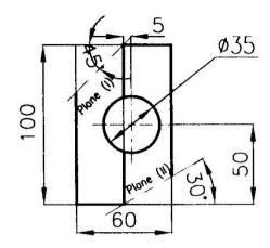
(b) Draw an isometric view of an object from the below given orthographic views.
