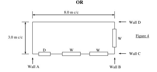
Figure 4 shows the plan of two storied brick masonry important building proposed at Zone III. Consider the thickness of wall A & B as 460 mm and of wall C & D as 340 mm. Decide the maximum size of windows for wall C considering width of door as 900 mm using IS: 4326 provisions. Also, enlist in detail with sketches, the necessary strengthening arrangements recommended for this building as per IS : 4326 provisions.
