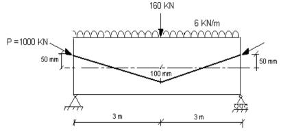
(b) A pretensioned member as shown in fig., 203 mm by 305 mm deep. It is eccentrically prestressed with 516 mm<sup>2</sup> of high tensile steel wire which is anchored to the bulkheads at unit stress of 1034 N/mm<sup>2</sup>. The c.g.s is 101.6 mm above the bottom fibre. The modular ratio is 6. Cmpute the stresses in the concrete immediately after transfer due to prestress only,using
