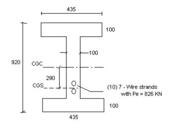
The properties of the sections are as follows  $A = 159,000 \text{ mm}^2$   $I = 1.7808 \text{ x } 10^{10} \text{ mm}^4$ .  $Ap = 960 \text{ mm}^2$ .
