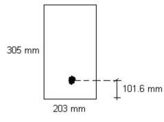
Q.3 (a) Design a simply supported (Type-II) pretensioned prestressed concrete beam for flexure only as per IS:1343-1980 with total moment  $M_T$ =435 kN-m (including an estimated self-weight moment  $M_{sw} = 55$  kN-m). The prestress at transfer is 1035 N/mm<sup>2</sup> and at service is 860 N/mm<sup>2</sup>.
