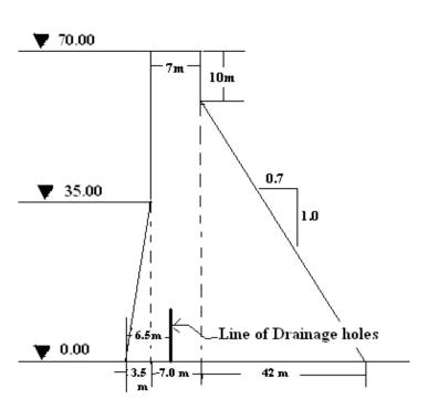
Fig.-1 Section of Gravity Dam Q-3(a)
