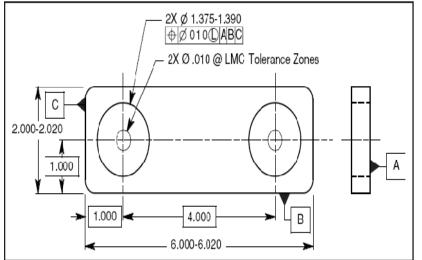
(b) Provide the appropriate datum feature symbols on the drawing and datums 06 in the feature control frames in below given fig. 6.
