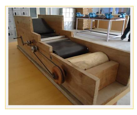
cost, semi-automatic and hand driven machine which may double the production capacity. The machine is ergonomically designed to mitigate back pain and other spinal problems. Using this machine, a woman may be able to roll about 6000 sticks a day.
