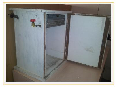
Team 2: The team from LDRP-ITR utilised this principle to develop a heat exchanger comprising network of pipes through which LPG gas can covered by thin and pass, spaced fins. The closely addition of fins help in effective faster cooling. and The insulating material helps in storing the cooling effect for a
