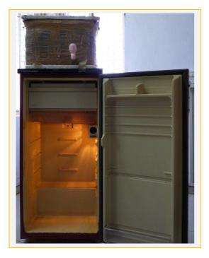
Modified Domestic refrigerator has two interesting novel functions. The waste heat of compressor is used to heat water, through a heat exchanger and in the process of removing heat, the life of compressor is extended and its efficiency goes up. Thus the power consumption also goes down because compressor has to work less.
