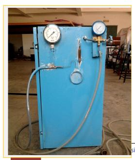
Team 1: The team from Laljibhai Chaturbhai Institute of Technology made a prototype in which the evaporator temperature reached -5  $^{\circ}$ C at an ambient temperature of 12  $^{\circ}$ C.
