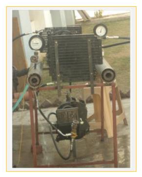
An automobile AC consumes about one-tenth of the total fuel. This is a significant cost for the vehicle owners such as truck drivers who travel round the clock running. It addresses this challenge by designing an AC that may be able to run itself by using waste heat from the automobile exhaust. It may therefore make the running of an automobile more economical.
